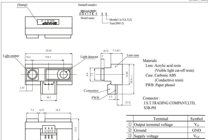
Note 1. The dimensions marked by "\*" show the dimensions of lens center position.
