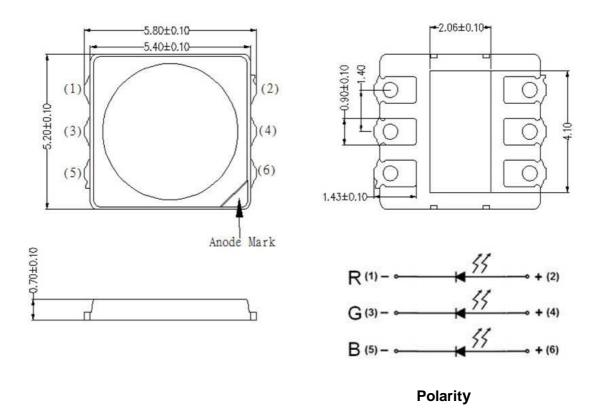
Unit: mm, Tolerance: ±0.1mm
