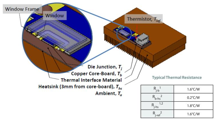
Note 1: Thermal resistance values are preliminary and are based on modeled results correlated to measured R<sub>j-hs</sub> data using the wavelength shift method. Verification of compliance with the recent releases of JEDEC Standards JESD51-14 and JESD51-5x series is pending.
