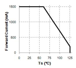
※Ts means soldering temperature
