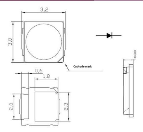
Unit: mm, Tolerance: ±0.1mm
