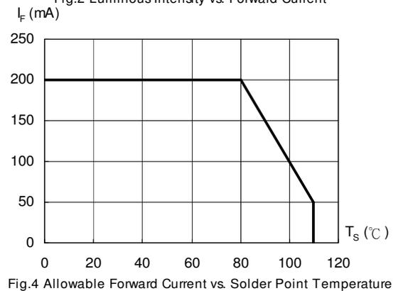
Fig.4 Allowable Forward Current vs. Solder Point Temperature
