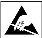
All LED materials, such as GaP, AlGaAs, AlInGaP, GaN, or InGaN chips, are STATIC SENSITIVE device. ESD protection or surge voltages shall be considered and taken care in whole product design and production processes.
