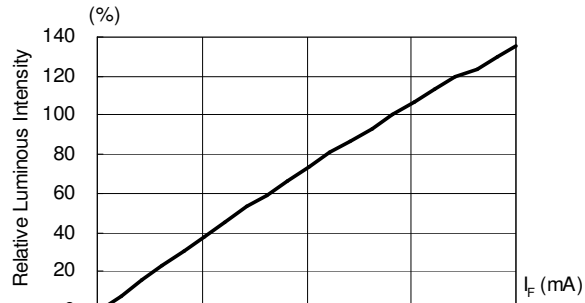
Fig.2 Luminous Intensity vs. Forward Current
