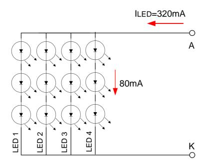
When LCM is operated over  $40^{\circ}\text{C}$  ambient temperature, the ILED should be follow :
