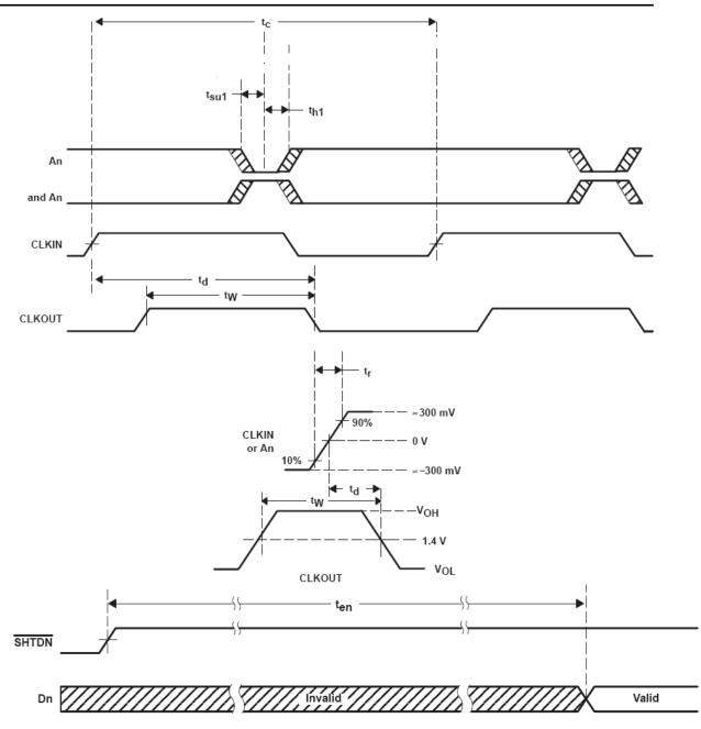
Figure 7. Enable Time Waveforms
