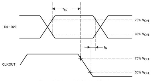
Figure 5. Setup and Hold Time Waveforms
