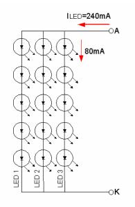
The constant current source is needed for white LED back-light driving.
