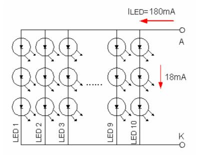
The constant current source is needed for white LED back-light driving. When LCM is operated over 60°C ambient temperature, the  $I_{BL}$  of the LED back-light should be adjusted to 135mA max
