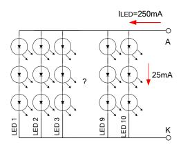
The constant current source is needed for white LED back-light driving. When LCM is operated over 60°C ambient temperature, the I<sub>BL</sub> of the LED back-light should be adjusted to 135mA max
