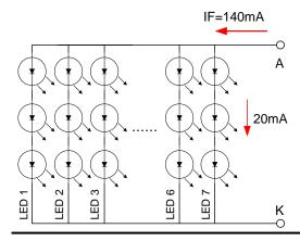
Note 6: When LCM is operated over  $60^{\circ}$ C ambient temperature, the I<sub>LED</sub> of the LED back-light should be adjusted to 105mA max
