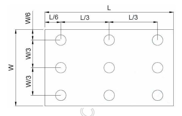
B<sub>max</sub>: The measured maximum luminance of all measurement position. B<sub>min</sub>: The measured minimum luminance of all measurement position.
