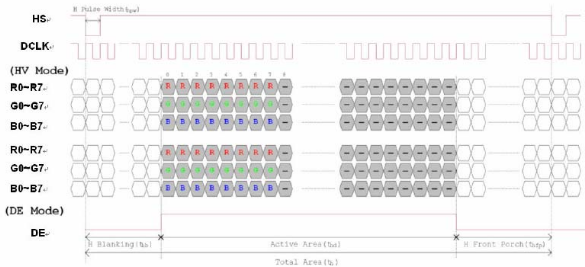
Figure 3. 1 Horizontal input timing diagram.
