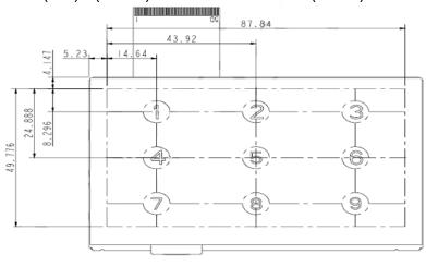
Fig.9-1: Test Point Position
