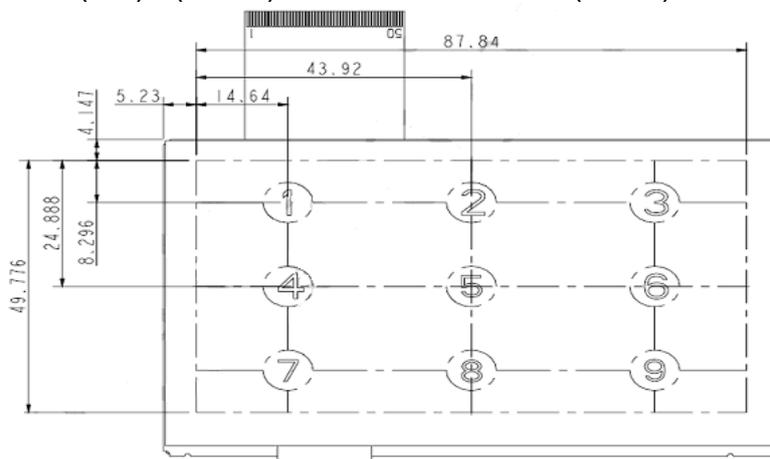
Fig.9-1: Test Point Position
