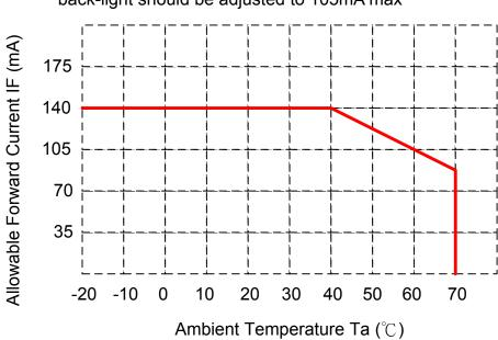
back-light should be adjusted to 105mA max
