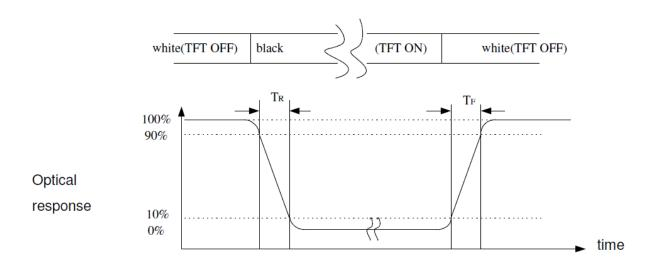
Note (4) Definition of optical measurement setup
