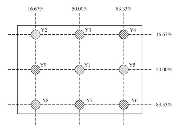
$\label{eq:Luminance of 9 points} \text{Luminance uniformity} = \frac{\text{(Min Luminance of 9 points)}}{\text{(Max Luminance of 9 points)}} \times 100\%$
