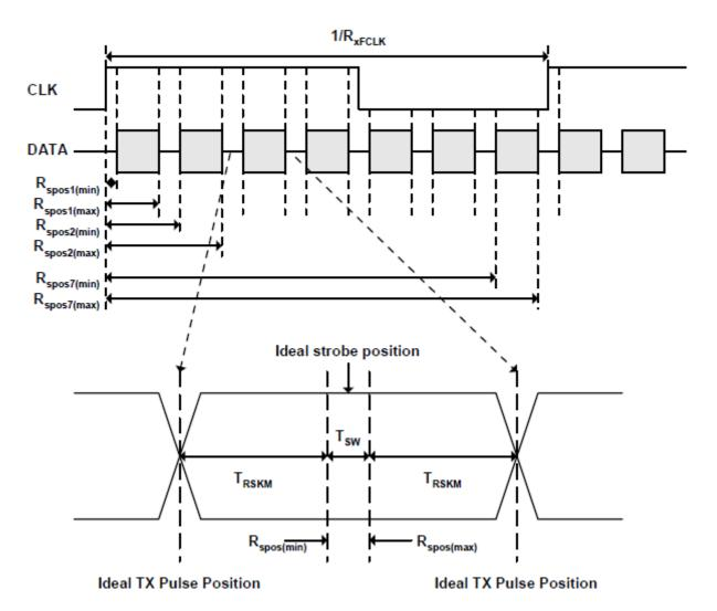
T<sub>RSKM</sub>: Receiver strobe margin R<sub>SPOS</sub>: Receiver strobe position T<sub>SW</sub> : Strobe width (Internal data sampling window)
