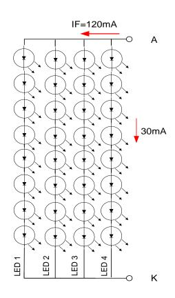
Note (3) When LCM is operated over  $40^{\circ}$ C ambient temperature, the IF should be follow :
