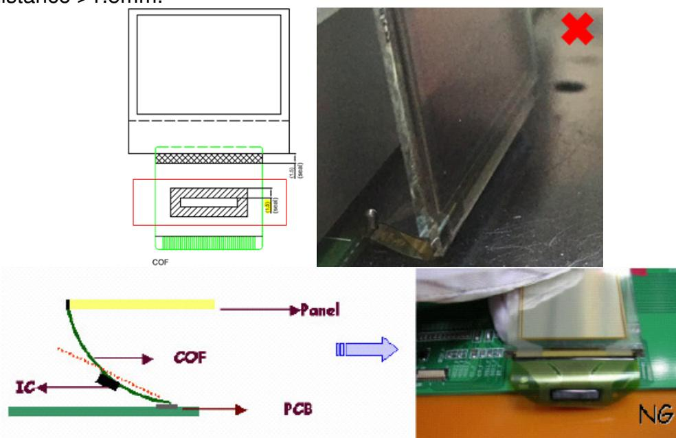
Use finger to insert COF /FPC into the connector when assembling the panel. Please refer to the photo.
