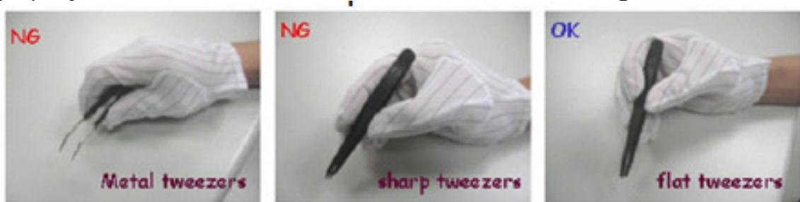
8. Please do not bend the film near the substrate glass. It could cause film peeling and TAB/FPC/COF damage. For TAB, It should bend the slit area as actual OLED it is. For FPC or COF, it is suggested to follow below pictures for instruction (distance between substrate glass and bending area >1.5mm; R>0.5mm).
