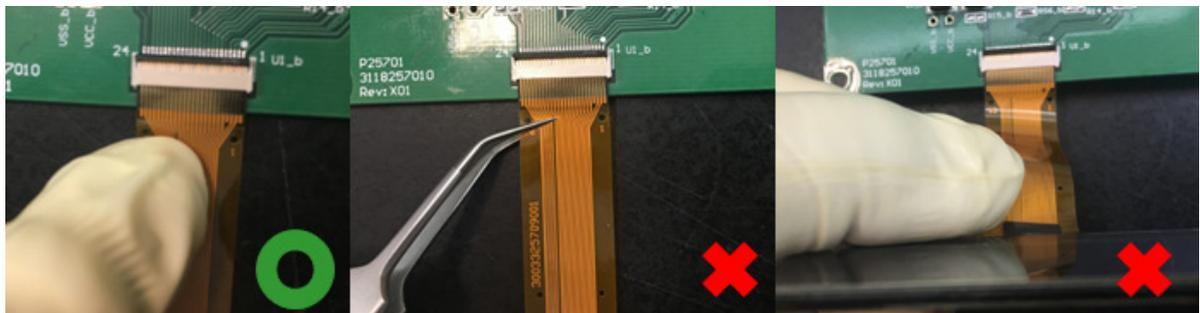
10. Do not wipe the pin of film and polarizer with the dry or hard materials that will damage the surface. When cleaning the display surface, use the soft cloth with solvent, IPA or alcohol, to clean.
