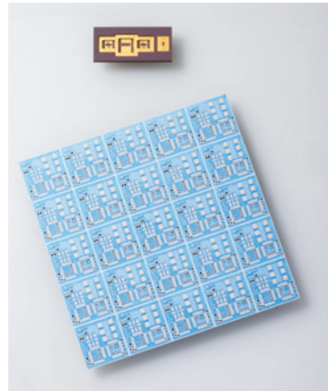
LTCC (Low Temperature Co-fired Ceramic) Substrate
